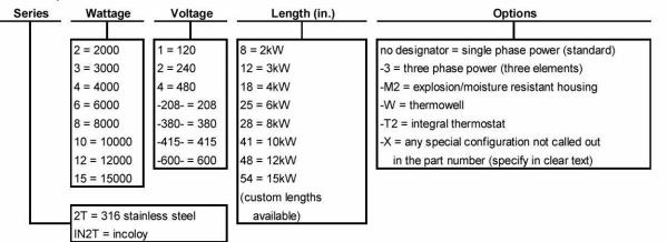
**T2T SERIES, 2" TITANIUM SCREW PLUG HEATER ORDERING INFORMATION**
